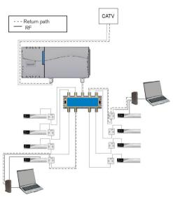
Example of an installation in a dwelling with 8 outlets. The CATV signals are distributed in each outlet.
