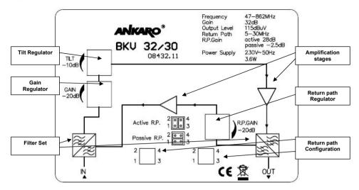
The gain of BKV 22/XX amplifier is 22dB for terrestrial band and 20dB for return path (active), for BKV 32/XX amplifier is 32dB for terrestrial band and 28 dB for return path (active).
